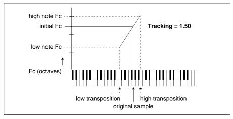
Use Filter Tracking to make the filter frequency follow the keyboard.
