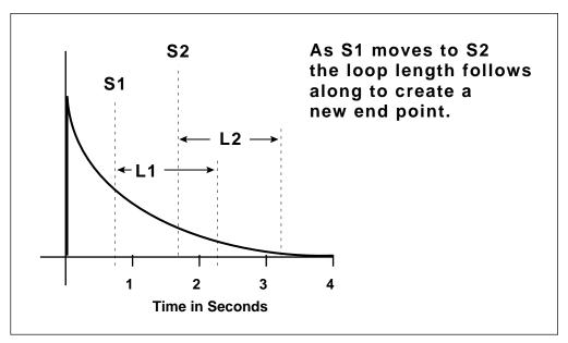
Moving the loop's Start Point adjusts the End Point of the loop as well.
