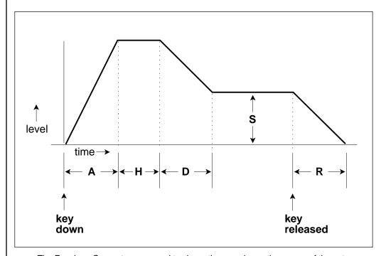
The Envelope Generators are used to shape the sound over the course of the note.
