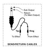
This diagram shows the type of cable used to access the Emax II submix sends and returns.
