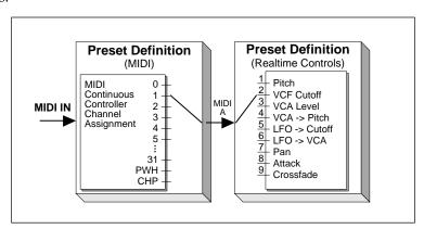
MIDI A and MIDI B can be thought of as "patchcords" which connect the MIDI Continuous Controller channels to the proper Realtime Control destination.
