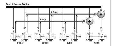
This diagram shows how the stereo jacks are used to function as effect sends and returns.
