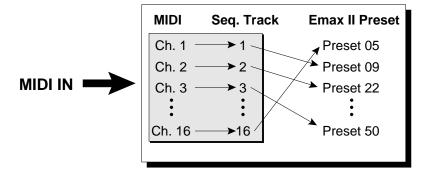
MIDI Channels are always routed to the same numbered Track. The Supermode Map directs a Track to the appropriate Preset. Emax II operation manual 181
