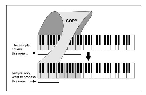
Copying a voice back to a subset of its former range gives you more voices that use the same samples. Using this technique, you could dynamically process each key separately if so desired.
