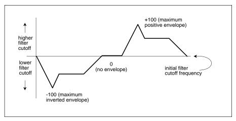
Inverted envelopes can be generated by applying a negative envelope amount.
