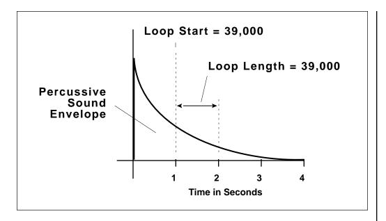
*Example:* If L reads L0039000, the loop is one second long at the highest sample rate. Select the parameter to adjust with the cursor buttons. Adjust the coarse value with the data slider and fine value with the increment and decrement keys, or enter a six-digit number. Loops have a minimum start point of 3 samples, and a minimum length of 32 samples.
