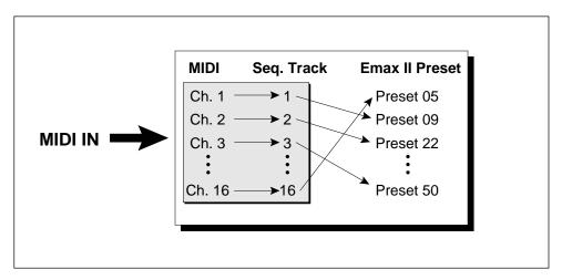
MIDI Channels are always routed to the same numbered Track. The SuperMode Map directs a Track to the appropriate Preset.
