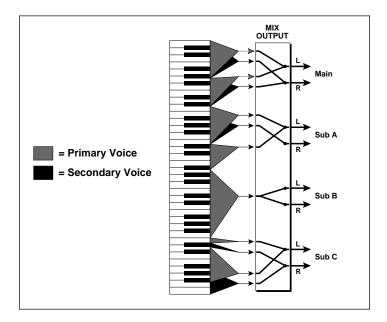
Groups of voices can be assigned to specific output channels using Dynamic Processing 21.
