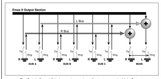
The Sub A, B, and C jacks can be used as effect returns to the Main Outputs.
