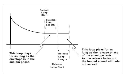
The Release Loop begins as soon as the key is released and continues until the sound fades out.
