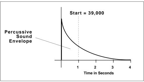
Adjusting the Truncation Start to 0039000, cuts one second off the beginning of the sample at the highest sample rate.
