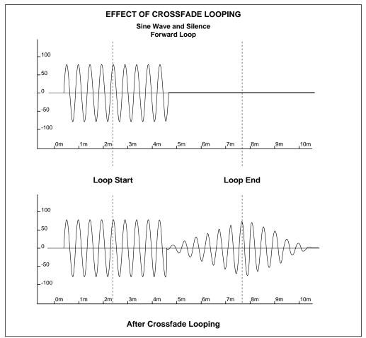
Crossfade Looping takes data from around the Start Point and fades it into the data from the End Point so that the data at both loop points is identical.
