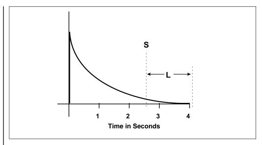
If the loop Length is at maximum (as occurs when you first call up a voice for looping), you cannot set a new S point since that would force the loop to "run out of sample". Shorten the Length before moving the S point.
